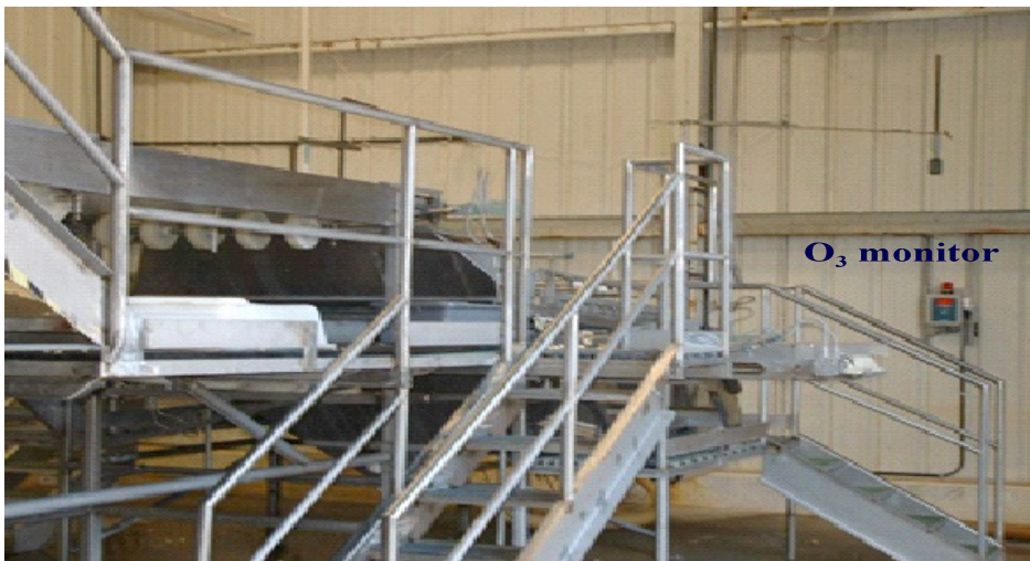
Conveyor system and ambient ozone monitor (mounted on wall to the right).
